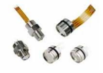
working technology to form Wheatstone bridge and precise mechanical structure, the measuring pressure is transmitted onto the silicon sensitive element through isolated diaphragm and filled silicon oil. This achieves the integrated high-accuracy transfer of the mechanical and electricity, the laser-trimmed thick-film resistors compensated temperature of the sensor.
